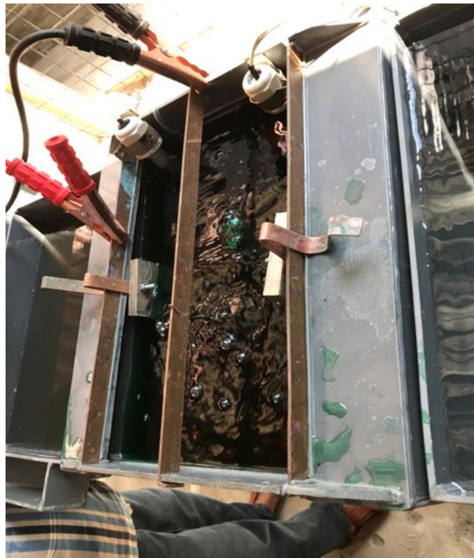
Gambar 3.36. Proses copper kilap plating
