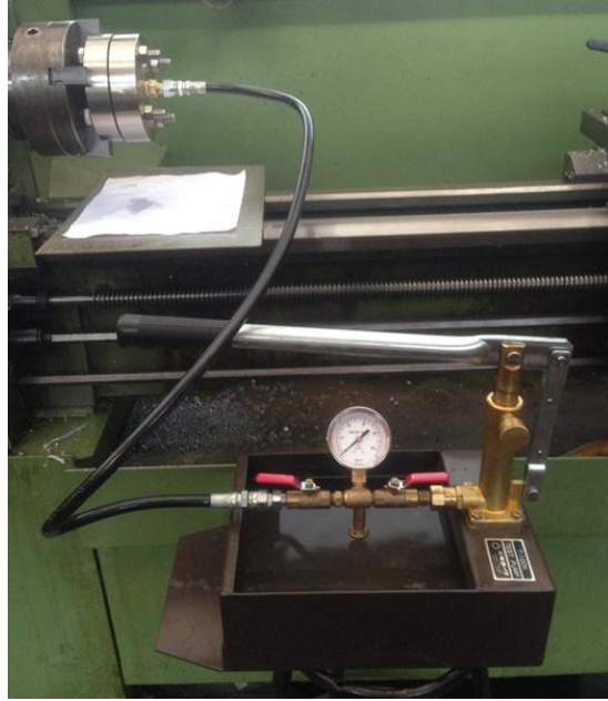
Gambar 3.13. Water pressure test
