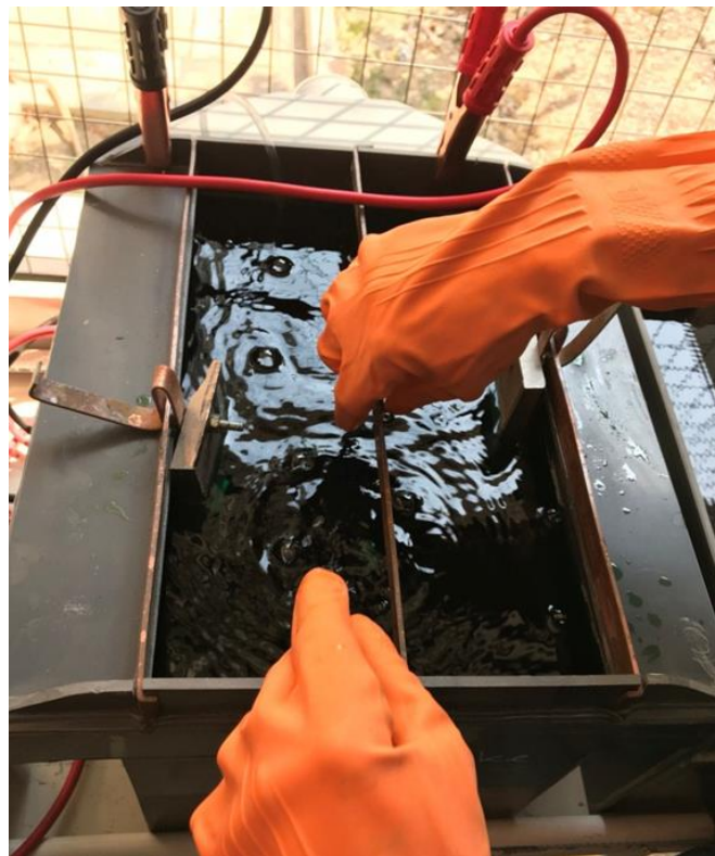
Gambar 3.32. Nickel strike plating
